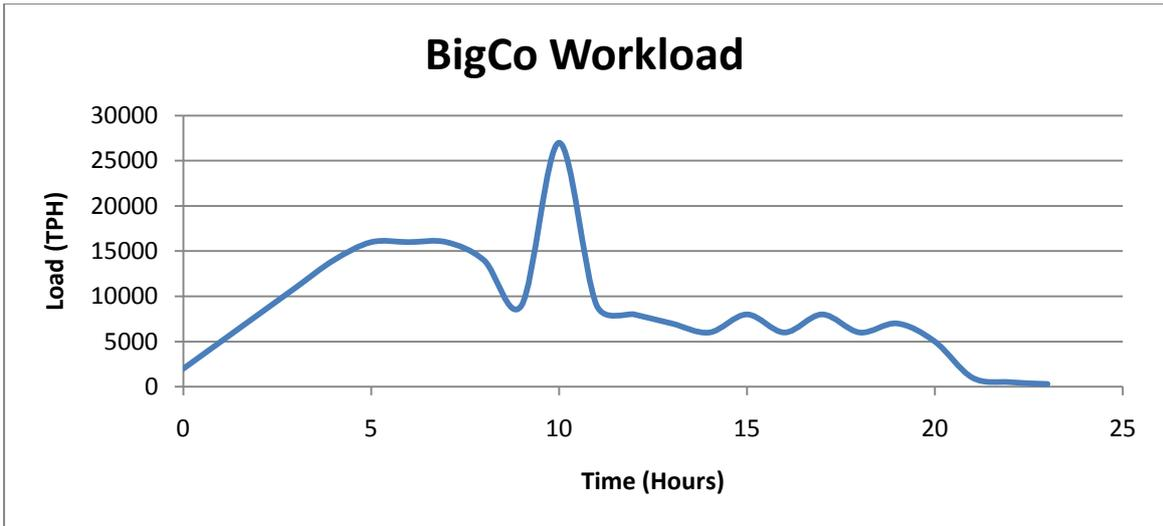
The next graph shows the percentage load change per hour, and reveals that there are two parts of the workloads that need rapid elasticity: The maximum peak at hour 10 with the maximum rate of increase per hour of 300%, but also the initial hour with 250%.
