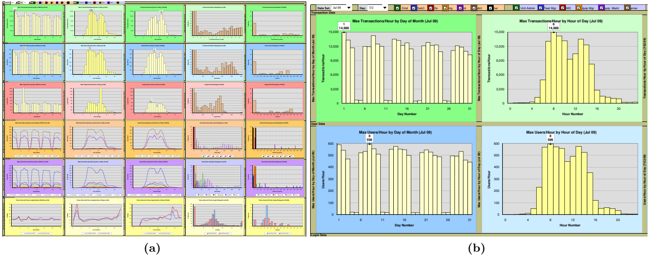
Figure 10: This figure shows a worksheet with 30 embedded charts. Chart (a) is a zoomed-out view. Chart (b) is a typical view. Outlining is used to control which charts are visible.
